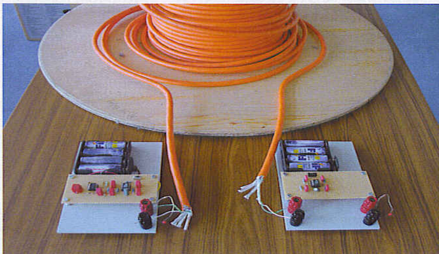
Figure 5. Test configuration with two LEDs to demonstrate the effect. A two channel scope can also be used in place of the LEDs.
